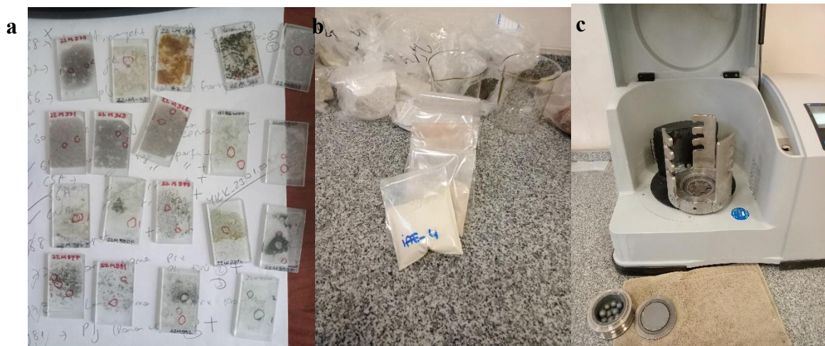
Figure 1. Preparation of petrographic a) thin sections, b) prepared samples, c) grinding machine
