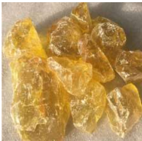
Figure 6 Glassy nuggets of rosin obtained from the process shown in Figure 5
