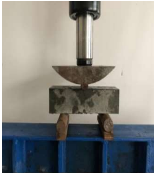
Fig 5. 3-Point Bending Test Setup [23]
