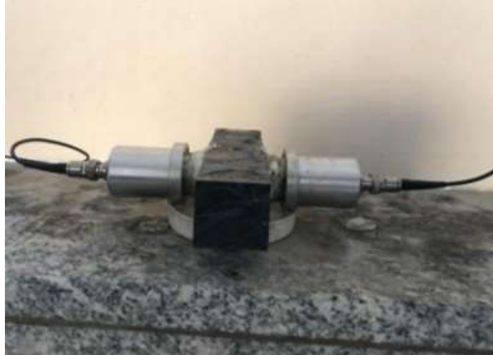
Fig 7 Set up of UPV test. [23]
