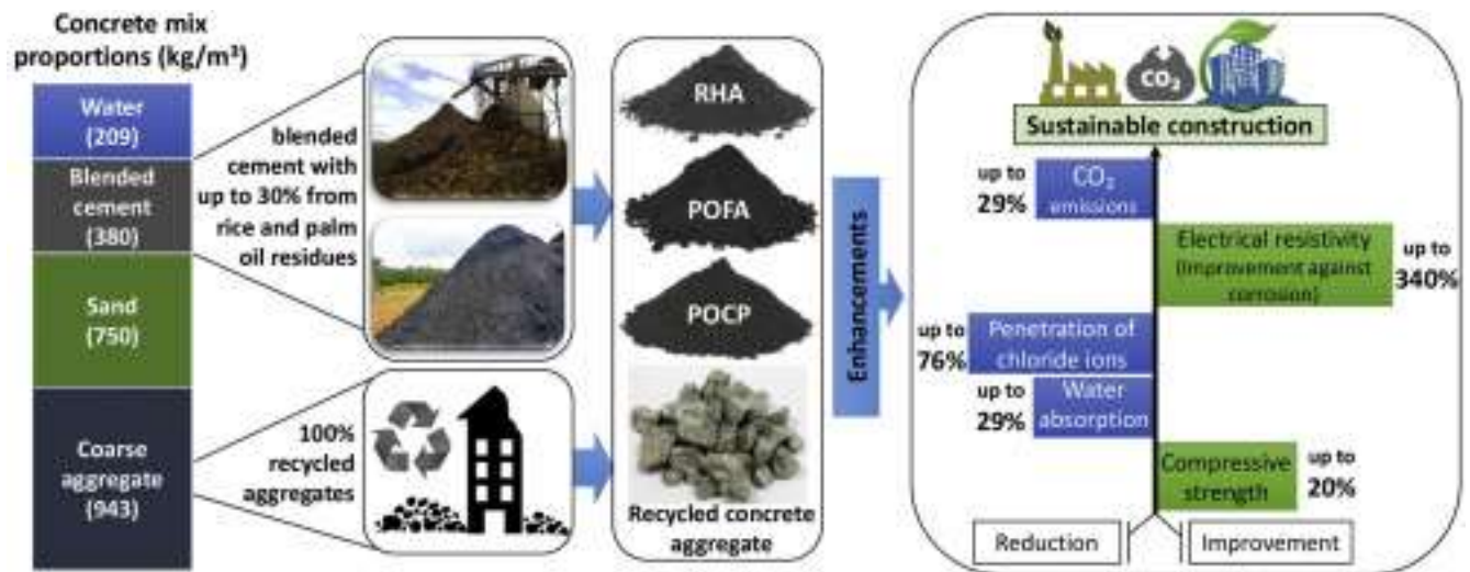
Fig 1. The use of waste materials in concrete production for a cleaner environment [3]
