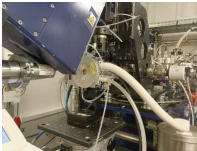
Figure 7 The Linkam heating stage mounted on the NCD-SWEET beamline at the ALBA Synchrotron Light Source. The blue box in the left hand top corner is the WAXS detector, just underneath it we can see the entrance tube to the vacuum chamber which reaches back to the SAXS Detector over 6m away to the left. The tubing connected to the stage is to enable cooling as well as heating control.
