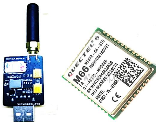
Fig. 6. GSM transceiver module using Quectel M66 chip
