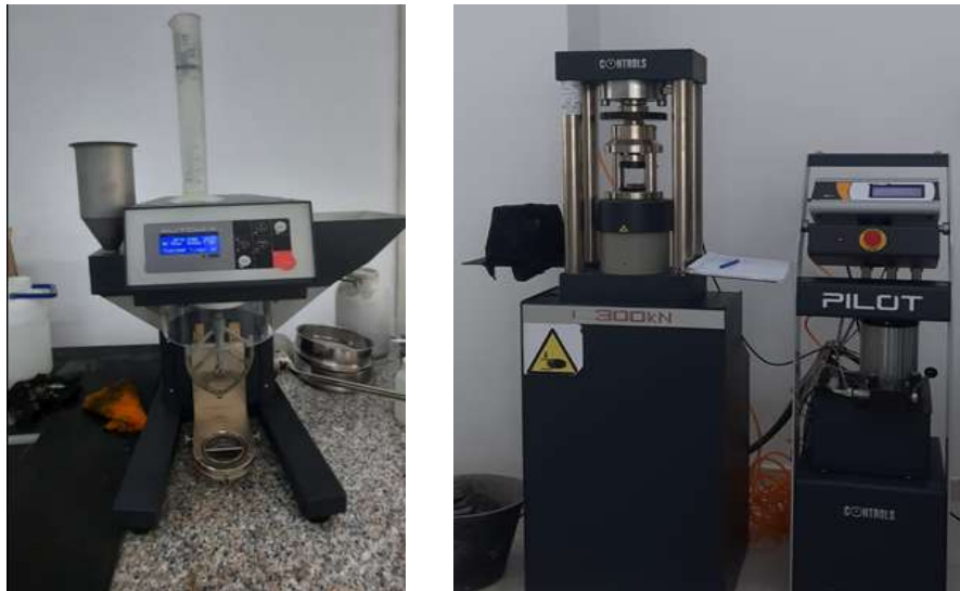
Fig. 6 a). Cement paste mixer and, b). Compressive strength apparatus (hydraulic press).
