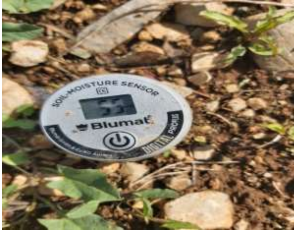
Figure 2 Tensiometer installed at the field
