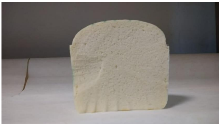
Figure 1. Internal view of bentonite-added polyurethane foam
